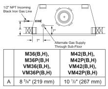
Figure 19 - Routing Incoming Gas Line
